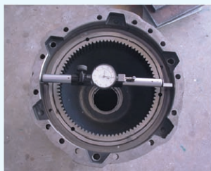
CYLINDRICAL MEASURING PINS FOR INTERNAL & EXTERNAL GEAR MEASUREMENT
